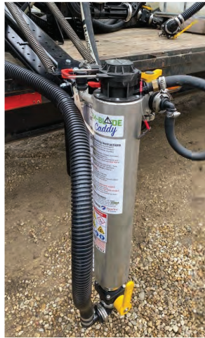
Swing Down configuration allows operator to work from ground
