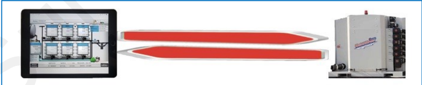
Red Lines = Connection FAILED (Login Credentials are incorrect)
