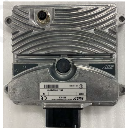
226-01-5319Y1 3CS Row Monitoring Sentinel ISOBUS ECU
