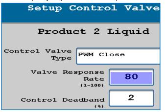
Start with the Valve Response Rate at 80. You will also make some changes in the Advanced Tuning (described later). If system is too slow to adjust to speed changes, increase Valve Response by 10 at a time. If the system overshoots and oscillates decrease by 10 at a time.
