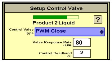
Start with the Valve Response Rate at 80. You will also make some changes in the Advanced Tuning (described later). If system is too slow to adjust to speed changes, increase Valve Response by 5 at a time.
