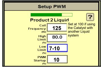
Start with the Low Limit and PWM Startup as shown above. Monitor the PWM DC % on the Run page. If the pump needs to go below 10% DC, change the Low Limit above. Adjust the PWM Startup % so the pump starts at the speed you want.
