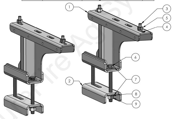
SureFire Accelerator (55, 110 and 155 gallon) or Catalyst™ (55 and 110 Gallon) tanks can be mounted above and offset from a toolbar using this z-mount bracket.
