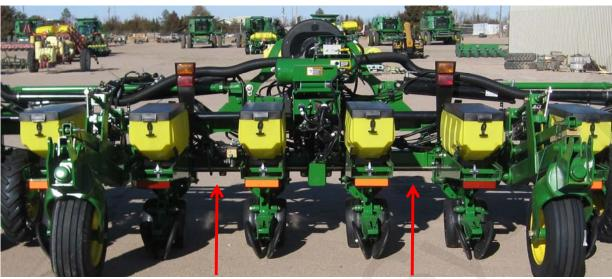
John Deere began mounting the electronics and air compressor on a mount in the very middle of the Model 1720 planter in late 2011. Between the seed boxes just right and left of center are two open locations where LiquiShift® Valve Stacks can be mounted. This bracket is designed to be installed in either of these locations.
