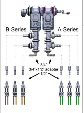
Feed section valves with 1-1/2" hose from pump. Each section valve may be split as necessary to feed the correct number of metering tube assemblies. (12 row example shown at left.)
