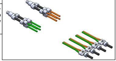
Mount flow indicators in banks (can be on one or multiple brackets). Dual metering tube Y's will attach to bottom of flow indicator. Top of flow indicator outputs through check valve to the row.
