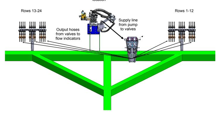
Valves A1 and B1 both feed the pre-assembled metering tube set which goes to the same set of flow indicators.
