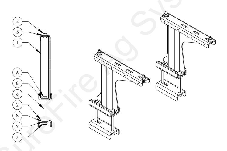
SureFire Accelerator (55, 110 and 155 gallon) or Catalyst<sup>M</sup> (55 and 100 Gallon) tanks can be mounted above and offset from a toolbar using this z-mount bracket. This kit attaches to 5" - 7" wide toolbars. The kit includes 3/4" x 9" bolts to work with a 7" tall bar.
