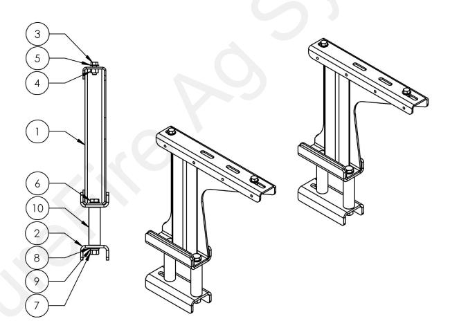
SureFire Accelerator (55, 110 and 155 gallon) or Catalyst™ (55 and 100 Gallon) tanks can be mounted above and offset from a toolbar using this z-mount bracket. The kits with spacer bushings are for toolbars that are 4" wide. The kit includes 3/4" x 8" bolts to work with a 5-6" tall bar with the use of a 5" or 6" tall spacer bushing.
