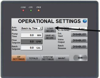
To navigate to the Load Recipe screen, press the LOAD RECIPE button on the Operational Settings screen.
