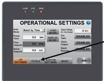
To navigate to the Totals screen, press the TOTALS button on any of the internal screens that have this menu shown.
