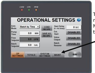
To navigate to the Maintenance screen, press the MAINT. button on any of the internal screens that have this menu shown.
