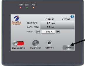
To navigate to the operational settings screen, press the SETUP button on the RUN screen.
