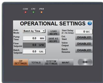
The SureBatch has three main modes of operation, and these are selected using the AUTO MODE drop down menu. The following table describes the operation of the three modes.
