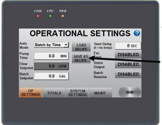
To navigate to the Save Recipe screen, press the SAVE AS RECIPE button on the Operational Settings screen.
