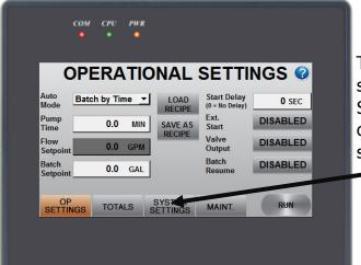
To navigate to the system settings screen, press the SYSTEM SETTINGS button on any of the internal screens that have this menu shown.
