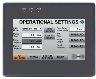
The START DELAY is used to delay the start of a batch by the number of seconds you enter. If this is set greater than 0, the system will wait for that amount of time after the batch is requested before the batch actually starts.
