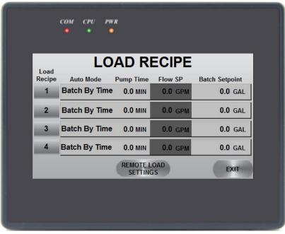
To LOAD RECIPE select the number button on the left hand side of the screen corresponding to the recipe that is desired to be loaded. Then a confirmation screen will be provided to verify the recipe to load. Loading a recipe will overwrite the existing AUTO MODE, PUMP TIME, FLOW SETPOINT, BATCH SETPOINT, and UNITS settings. Then you can use the START/STOP or remote key fob to control the batch.
