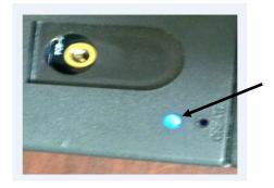
**Step 3:** While blue light is flashing turn remote over then starting from bottom left push the numbers in numerical order 1 through 8. Number 1 on this remote is the start, button 2 is stop, 3 is above the start button, 4 is above stop, 5 is R3, 6 is R4, 7 is R1 and 8 is R2. Buttons 1-8 must be pushed in numerical order while the blue light flashes. This will create a code for the remote.
