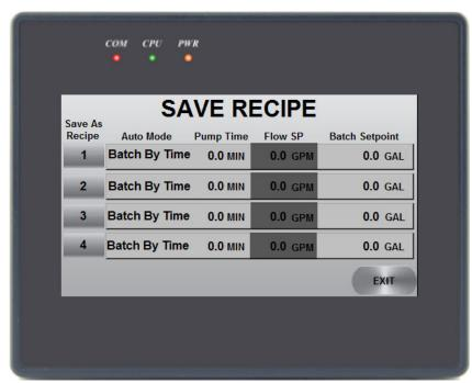
To SAVE RECIPE select the number button on the left hand side of the screen corresponding to the recipe that is desired to be saved. Then a confirmation screen will be provided to verify the recipe to save. Saving a recipe will overwrite the existing AUTO MODE, PUMP TIME, FLOW SETPOINT, BATCH SETPOINT, and UNITS settings for the recipe number you select. Going to the LOAD RECIPE screen is a good way to verify that the recipe has been saved correctly.
