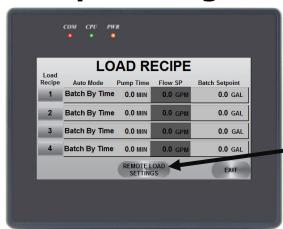
To navigate to the Remote Load Settings screen, press the REMOTE LOAD SETTINGS button on the Load Recipe screen.
