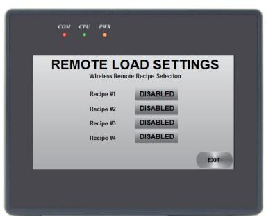
The REMOTE LOAD SETTINGS screen controls which recipes can be loaded using the key fob remote. These settings effectively enable or disable the R1-R4 buttons on the remote control. For example, if Recipe #1 is enabled, then when the R1 button is pressed on the remote, the recipe settings for recipe 1 will be loaded and the batch will start. Also, if Recipe #2 is disabled on this screen, then pressing the R2 button will do nothing.
