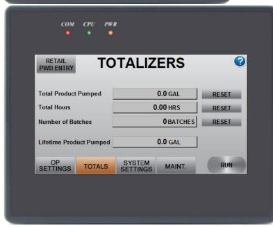
This screen keeps track of several useful totalizers. TOTAL PRODUCT PUMPED is an end customer resettable totalizer that can be used to get a combined total of several batches.
