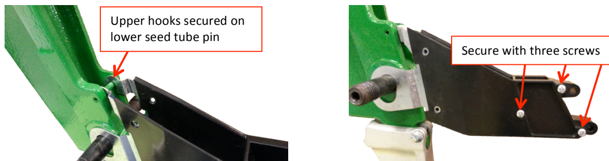
Illustration 2 – Quick Attach Keeton Firmer Bracket Installed
