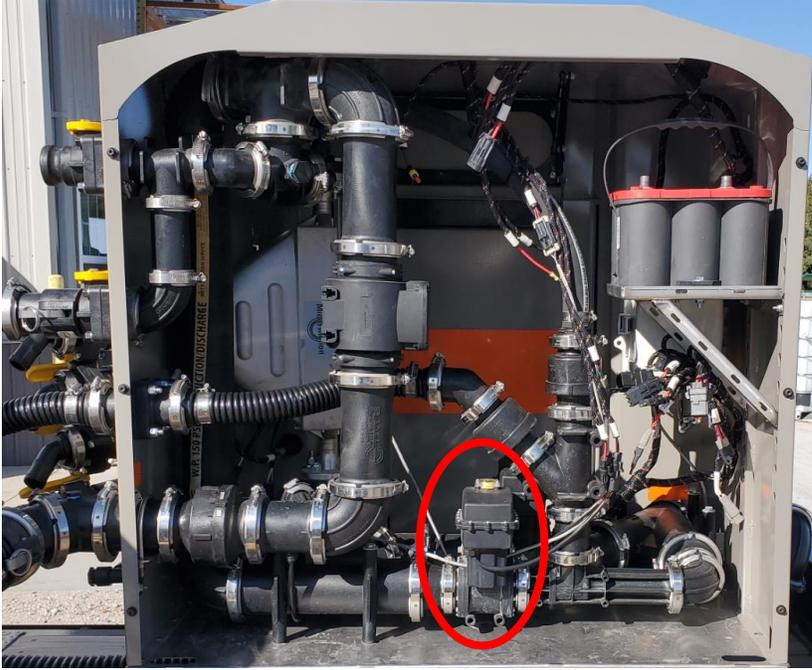
Picture shows modified plumbing. Note the new valve and venturi location.
