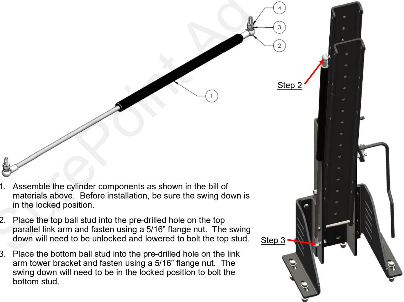
1. Assemble the cylinder components as shown in the bill of materials above. Before installation, be sure the swing down is in the locked position.
