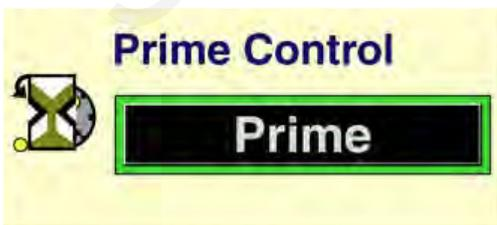
The Prime Control window is used to prime the seed meters and liquid fertilizer system.
