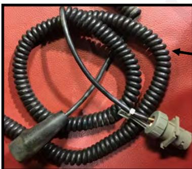
Tether switch from Case. Connects to connector on back of planter (Jump across these two pins on planter connector to activate pump without tether switch)
