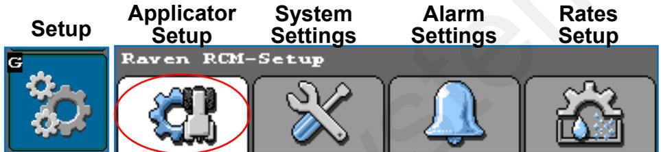
For the initial setup, start a new profile. The Raven RCM allows you to store 8 profiles. Be prepared to wait during this phase of the setup process.
