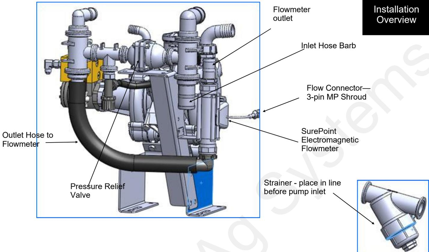
**Inlet:** The D160 and D250 PumpRight is shipped with a 2" inlet hose barb. Attach this to the hose from your supply tank and strainer. A 2" 90 degree hose barb is included and can be substituted.
