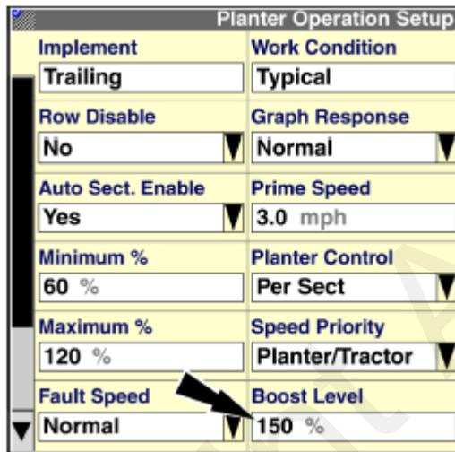
**Boost Level** determines the startup boost level for the liquid fertilizer pump. This is a 4-second boost on startup to fill the lines and get to target rate. 150% is a good starting point. With this setting, the controller briefly brings the pump to 150% of the target rate and then returns to the target. Adjust as desired in the field.
