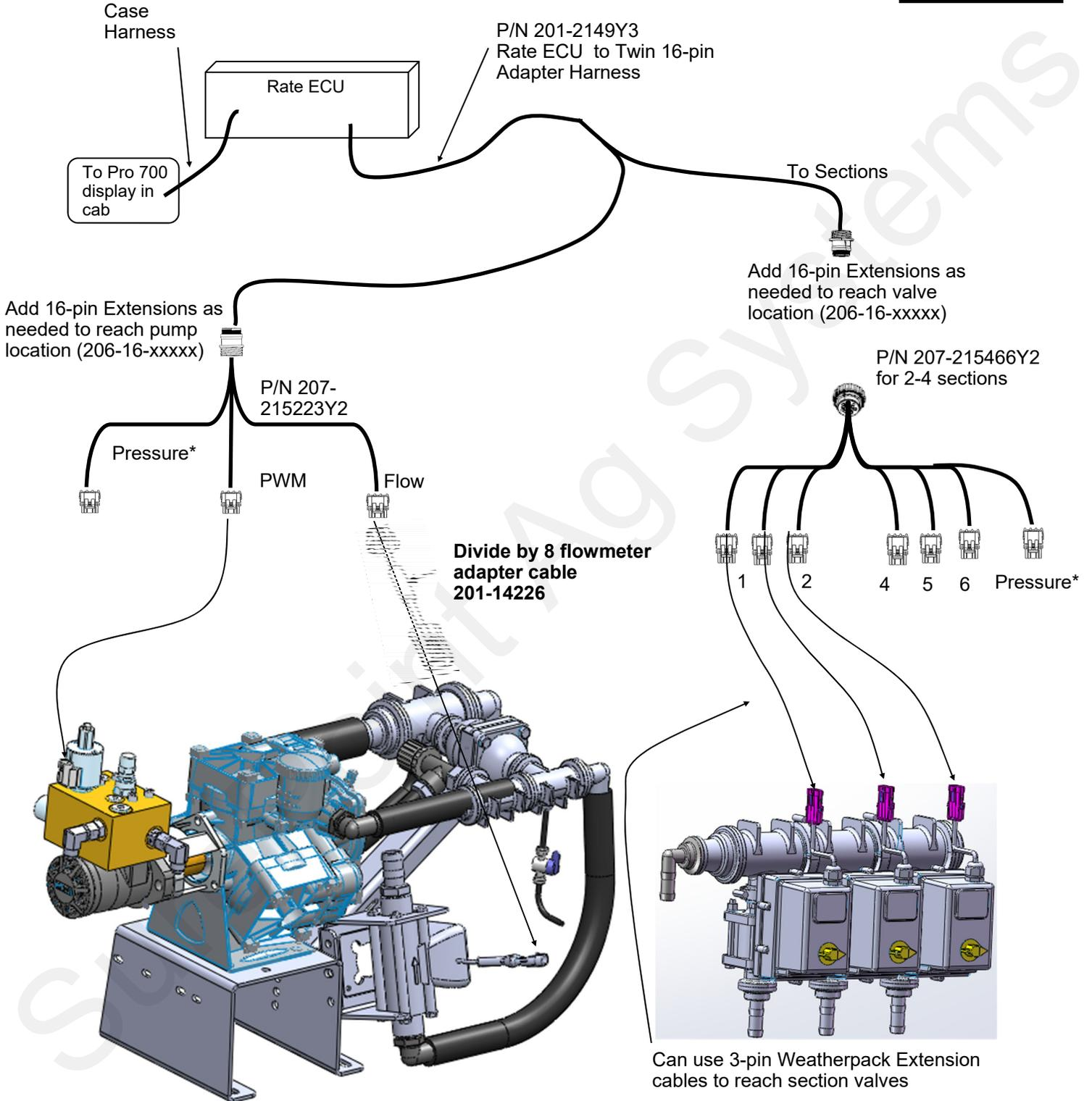
\* At this time, the liquid pressure sensors are not available for the Pro 700 Planter ECU system.
