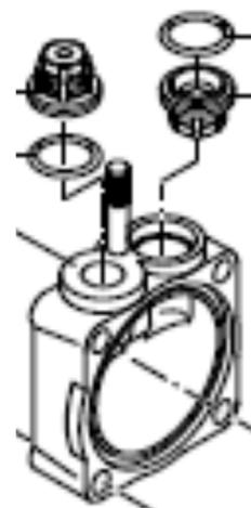
D70 - D115 Valves are on same side of head. Valves should pop out with slight screwdriver pressure.
