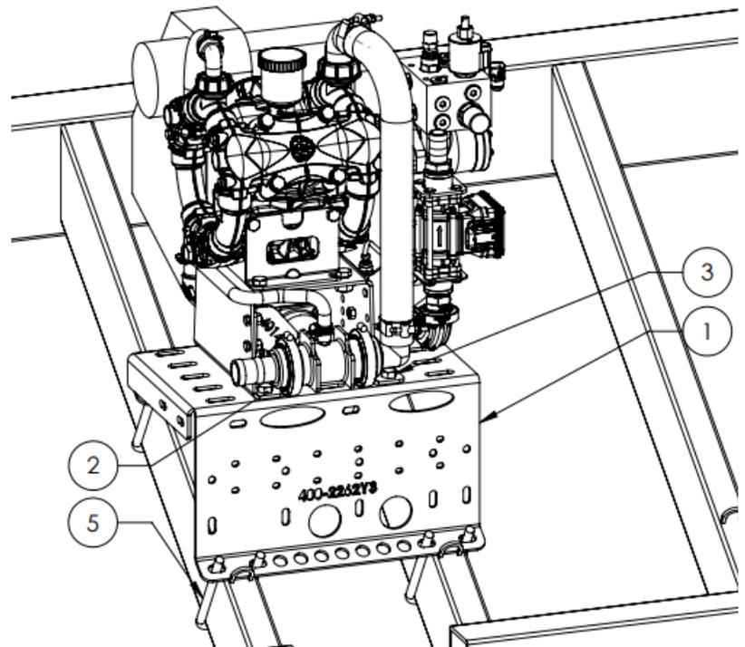
Use four (4) 1/2" x 1" hex head bolts and flange nuts to mount PumpRight pump unit to 400-2262Y3 bracket.
