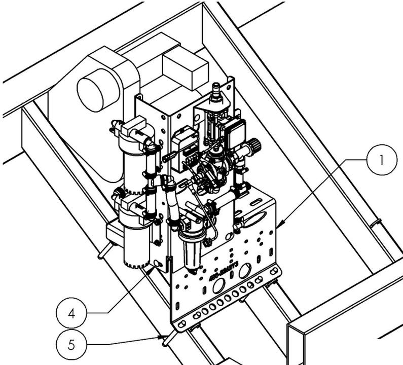
Use four (4) 3/8" x 1" carriage bolts and flange nuts to mount Tower or Odyssey pump to 400-2262Y3 bracket.
