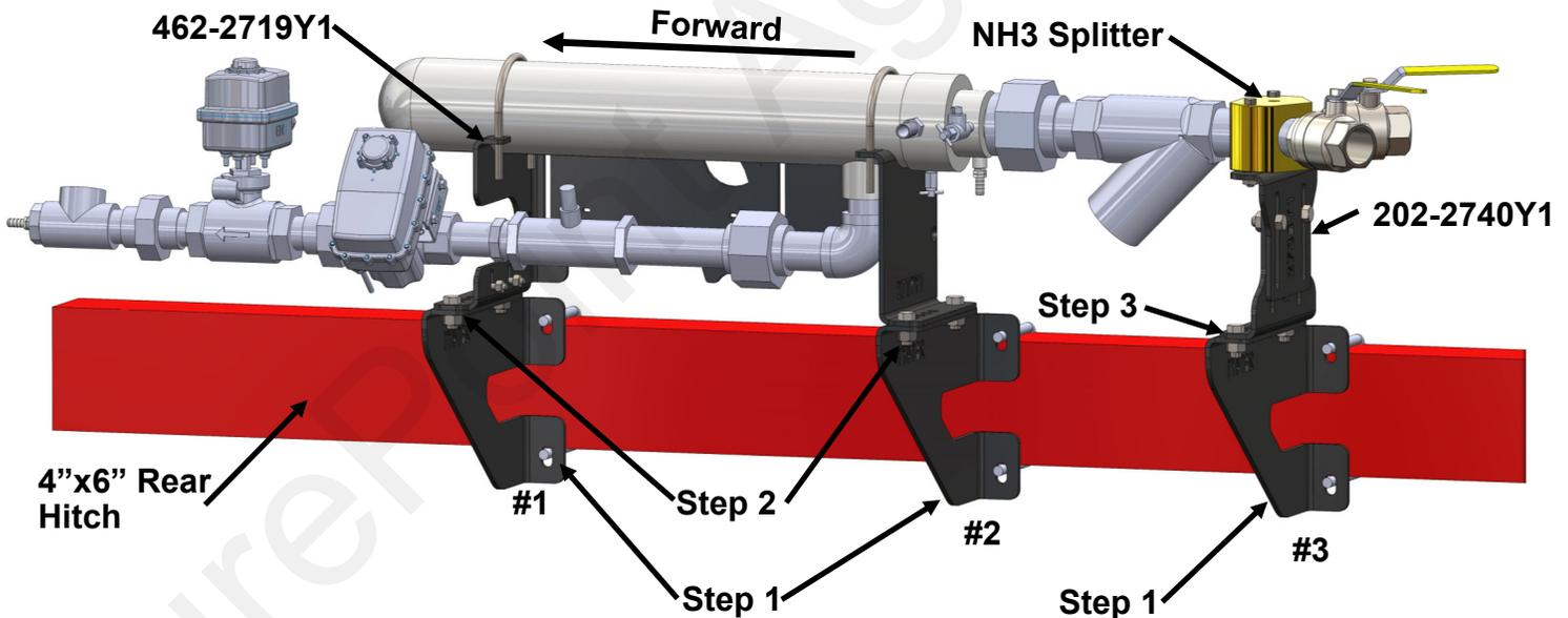
1. Mount all three Offset Brackets to the 4"x6" Rear Hitch Bar using the provided 1/2"x6"x5" Square Bent U-bolts (380-1017). Brackets #1 and #2 should be approximately 23 inches apart. Bracket #3 should be approximately 16-1/2" from Bracket #2. Do not fully tighten to allow for adjustment in Steps 2 & 3 .
