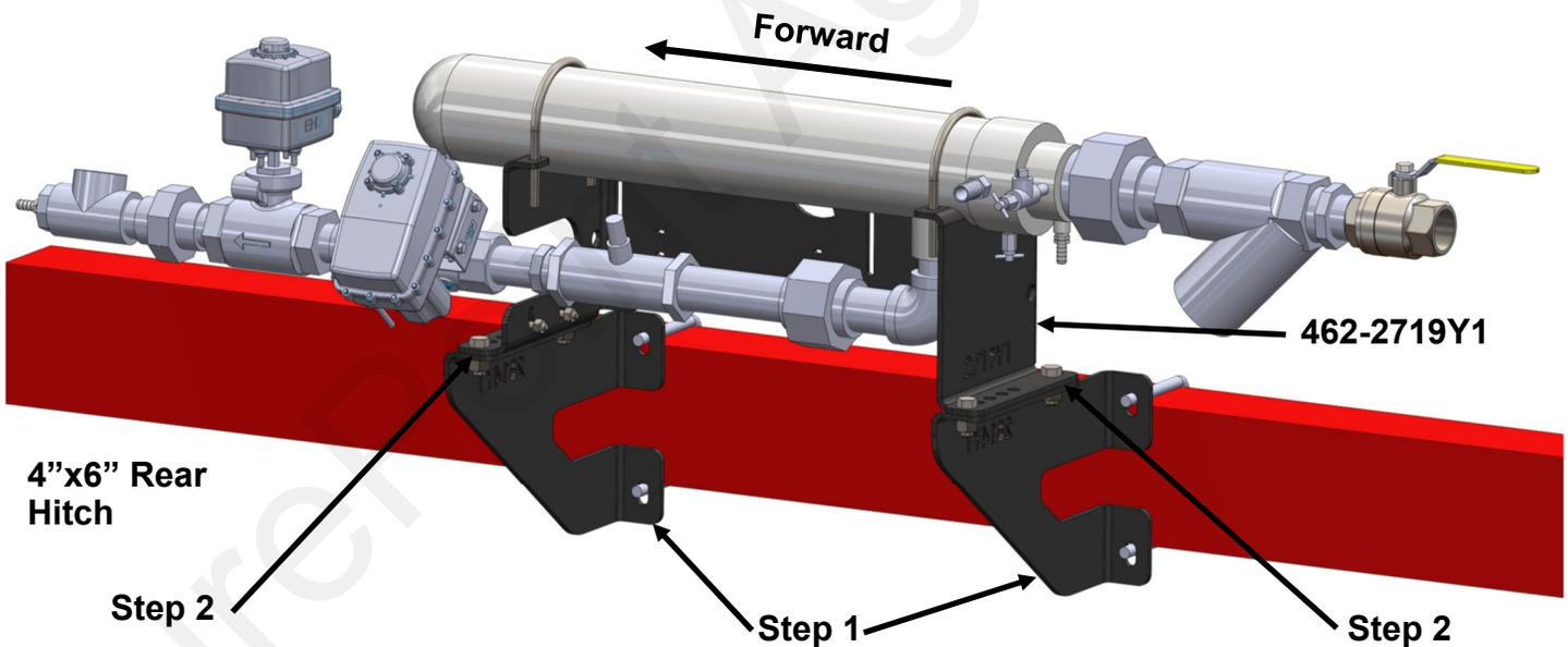
1. Mount both Offset Brackets to the 4"x6" Rear Hitch Bar using the provided 1/2"x6"x5" Square Bent U-bolts (380-1017). The Brackets should be approximately 23 inches apart. Do not fully tighten to allow for adjustment in Step 2.
