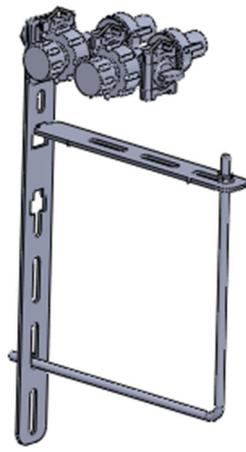
**Example 3.** Use the long bracket on the front of a 3x7 bar (vacuum tube on some planters). Mount the check valve hanging forward of the bar. The supply line will run directly over the bar. The excess bolt and bracket length can be cut off.
