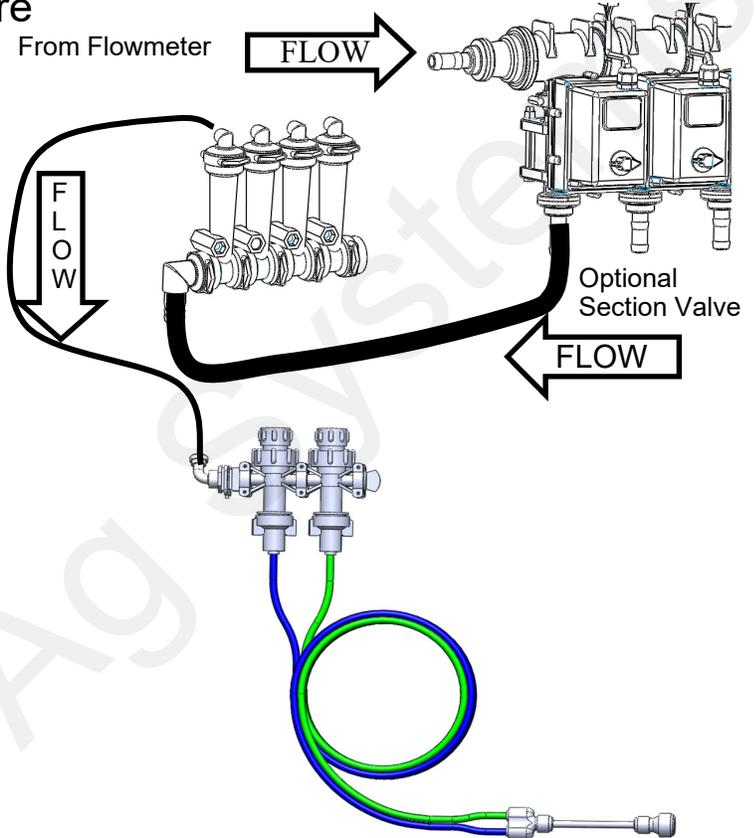
**SurePoint dual metering tube plumbing kits** are a great way to plumb a planter to apply starter fertilizer or high rate applications. They'll also work on other implements when applying low or high rates of fertilizer.
