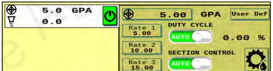
Toggle between Rate 1, 2, and 3 on the go, or press the top Target Rate box and enter a different target. Press the gear/teardrop on the bottom right to go to the Rate Setup screen.
