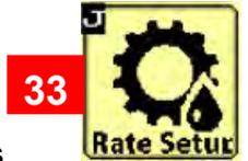
34.) **Flow Adjustment** - Use this to synchronize the Sentinel flowmeter modules with the main system flowmeter. Once the accuracy of the main flowmeter has been confirmed, change the Flow Adjustment factor as needed to synchronize the Sentinel reading with the main flowmeter reading.
