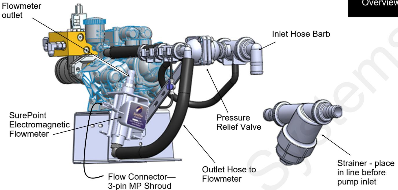
**Inlet:** The D70 and D115 PumpRight is shipped with a 1 1/2" inlet hose barb. Attach this to the hose from your supply tank and strainer . A 1 1/2" 90 degree hose barb is included and can be substituted.
