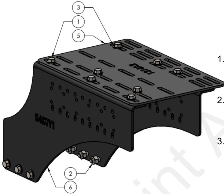
1. Mount 400-5467Y1 to the support plate using three (3) 1/2" x 1-1/2" hex head bolts, washers, and nuts
