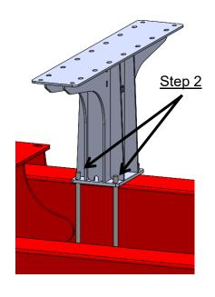
2. Loosely mount pedestal 421-2424Y2 clear of the gusset on the hitch using the hardware provided in kit 380-1067.
