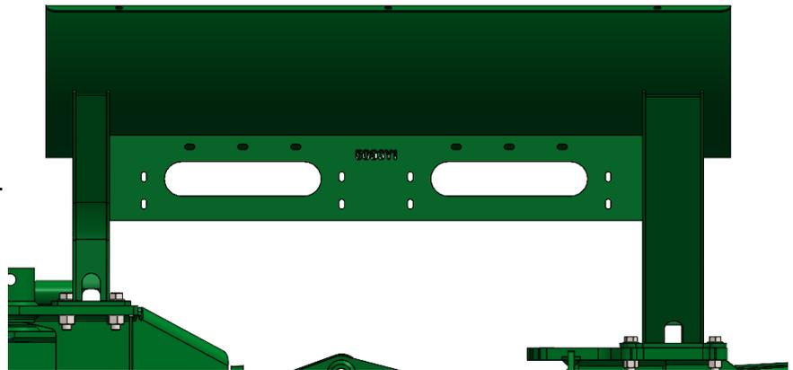
4. Finally, install the tank in the saddles and fasten the tank strap mounting brackets, and tank straps. Check for clearance from seed boxes when folding and when the drill is raised and lowered. Note: Tighten straps again once the tank has been filled.
