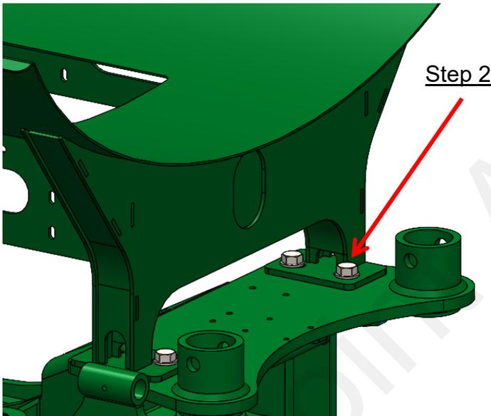
2. Loosely mount the back of 450-5093Y1 - 400 Gallon Tank Bracket to the bolt plate on the hitch using four (4) 3/4" x 2-1/2" hex head bolts, washers and flange nuts.
