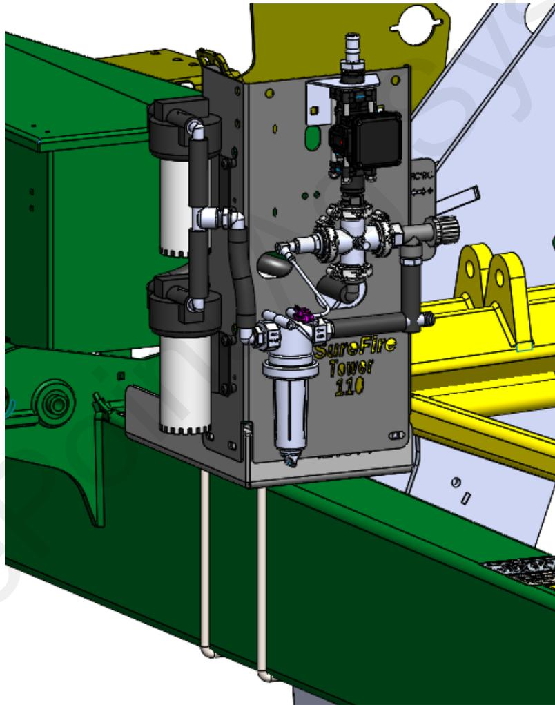
1. Mount 410-4213Y1 tower mounting bracket to the hitch using two (2) 1/2" x 6" x 12" U-bolts. (Two 6" x 18" u-bolts for BD7600-40 will not be used)
