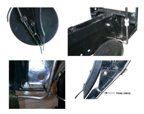
Install hose clamp around the shank and placement tube, just above the inside disc scraper. This will hold the tube against the bottom of the shank.
