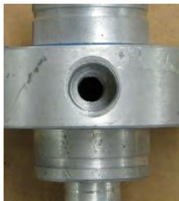
Threaded orifice not installed
