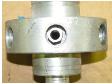
Threaded orifice installed
