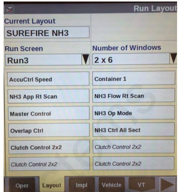
The Run Screen Layout is largely a matter of operator preference. Some of these items may be added to the Left Hand Area if space is available there or more than one Run Screen can be set up.
