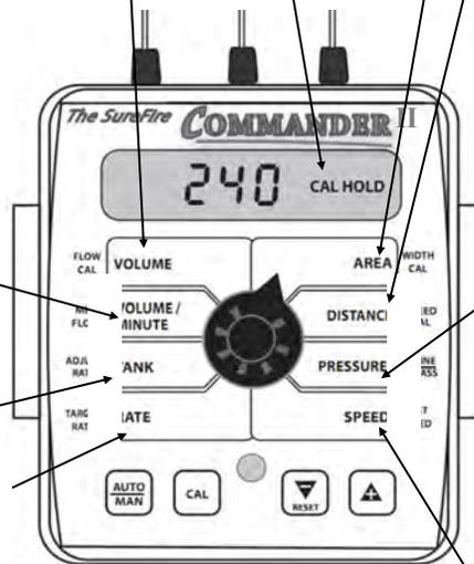
**CONTROL SPEED:** Typically -2 for PumpRight Hydraulic Pumps.
