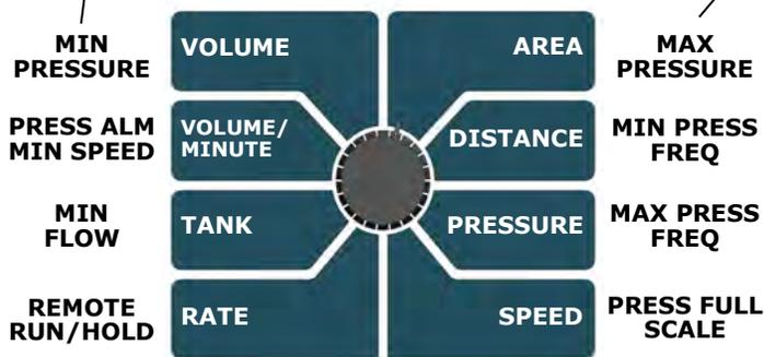
**MIN FLOW:** The purpose of this calibration value is to prevent the system from applying below the recommended minimum rate for spray nozzles.
