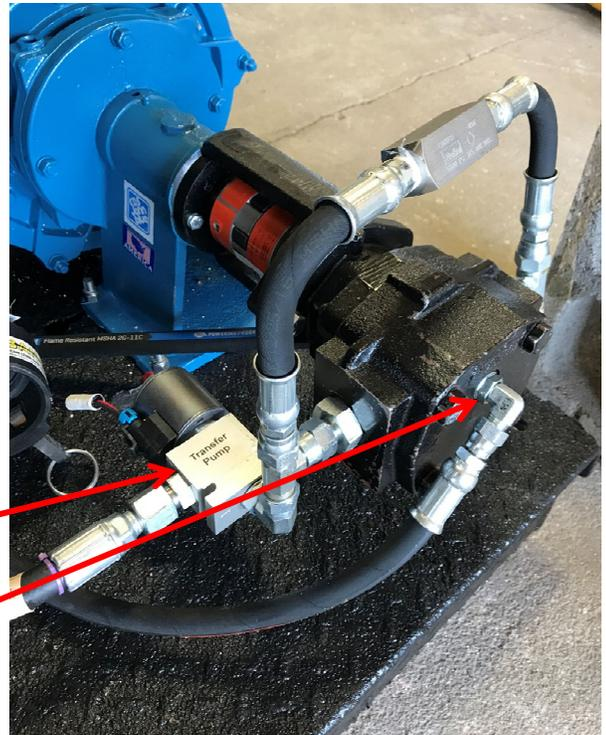
Transfer Pump Solenoid Valve Assembly
