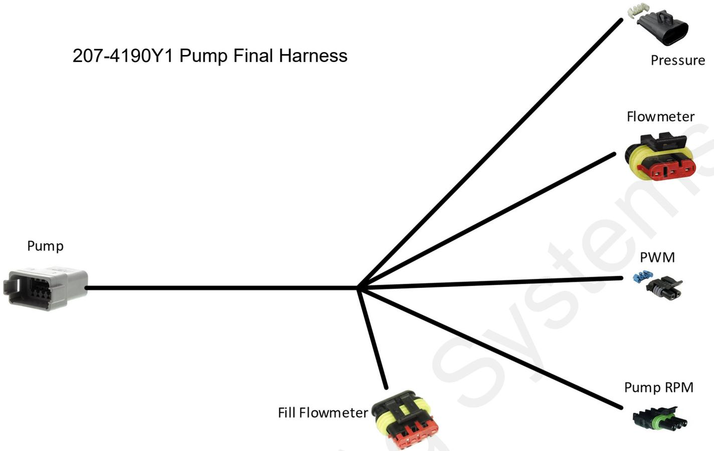
*Note: On the Trimble Field-IQ module, the Pump Final harness MUST have a Yellow and a **Green** wire on the PWM connector. 207-3461Y2 will NOT work.*
