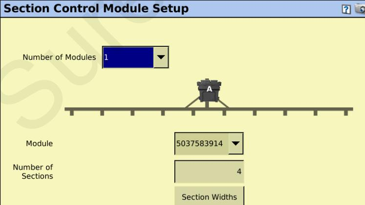
The screenshot shows a 'Section Control Module Setup' window. At the top is a dropdown menu for 'Number of Modules' set to '1'. Below is a diagram of a horizontal bar with several vertical tick marks and a central module labeled 'A'. Below the diagram are three input fields: 'Module' (dropdown menu with '5037583914'), 'Number of Sections' (text box with '4'), and 'Section Widths' (text box).
