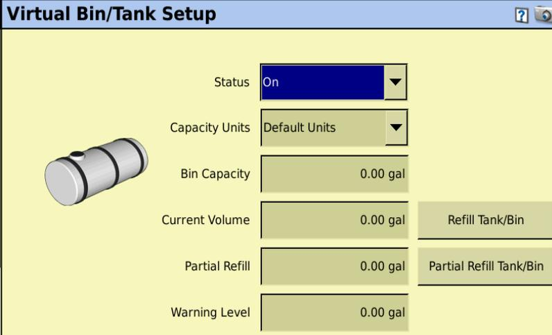
The screenshot shows a 'Virtual Bin/Tank Setup' window. On the left is a 3D rendering of a cylindrical tank. To its right are several input fields: 'Status' (dropdown menu set to 'On'), 'Capacity Units' (dropdown menu set to 'Default Units'), 'Bin Capacity' (text box with '0.00 gal'), 'Current Volume' (text box with '0.00 gal' and a 'Refill Tank/Bin' button), 'Partial Refill' (text box with '0.00 gal' and a 'Partial Refill Tank/Bin' button), and 'Warning Level' (text box with '0.00 gal').
