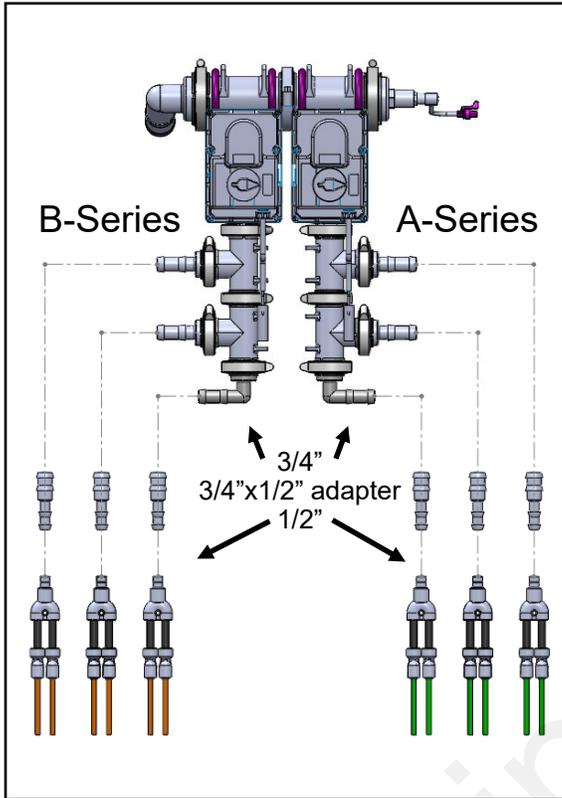
Feed section valves with 1-1/2" hose from pump. Each section valve may be split as necessary to feed the correct number of metering tube assemblies. (12 row example shown at left.)
