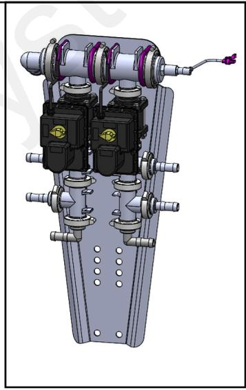
Dual metering tube comes pre-assembled. Hose barb ends go to section valves, 3/8" tubing goes to flow indicators.
