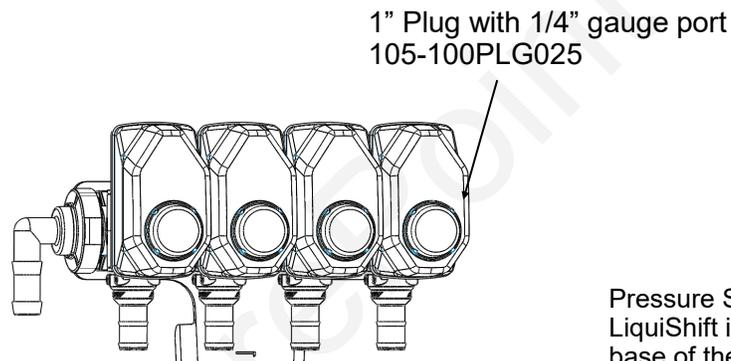
Pressure Sensor for LiquiShift is mounted at the base of the valve stack. The same sensor is used for LiquiShift and displayed on the display.
