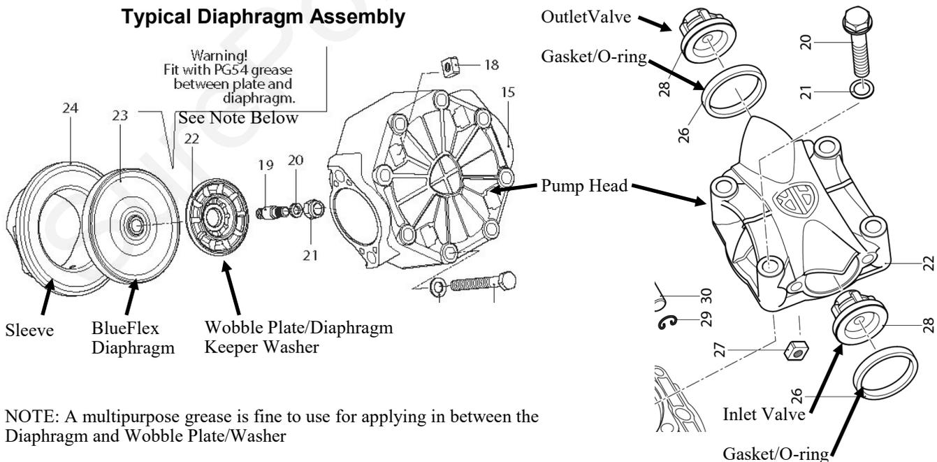
**NOTE: A multipurpose grease is fine to use for applying in between the Diaphragm and Wobble Plate/Washer**
