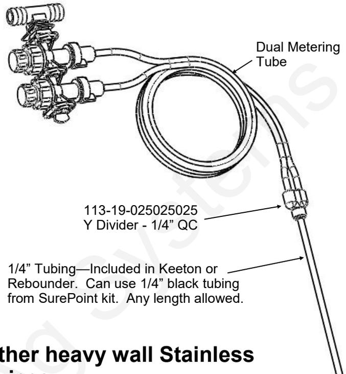
For thin wall stainless steel tubes, you can push the 1/4" black tubing all the way through the stainless steel tube so fertilizer will run directly from the tubing onto the ground.
