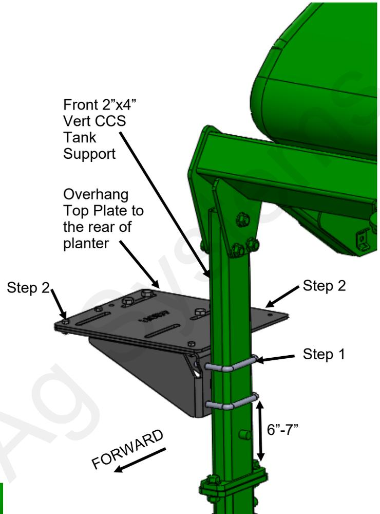
3. Mount the LiquiShift Valve Stack on bracket as shown to the left using the supplied 1/2" Hardware. Make sure the valve stack is mounted to the rear of the support bracket. If this is not the case, collision when folding planter could become an issue.
