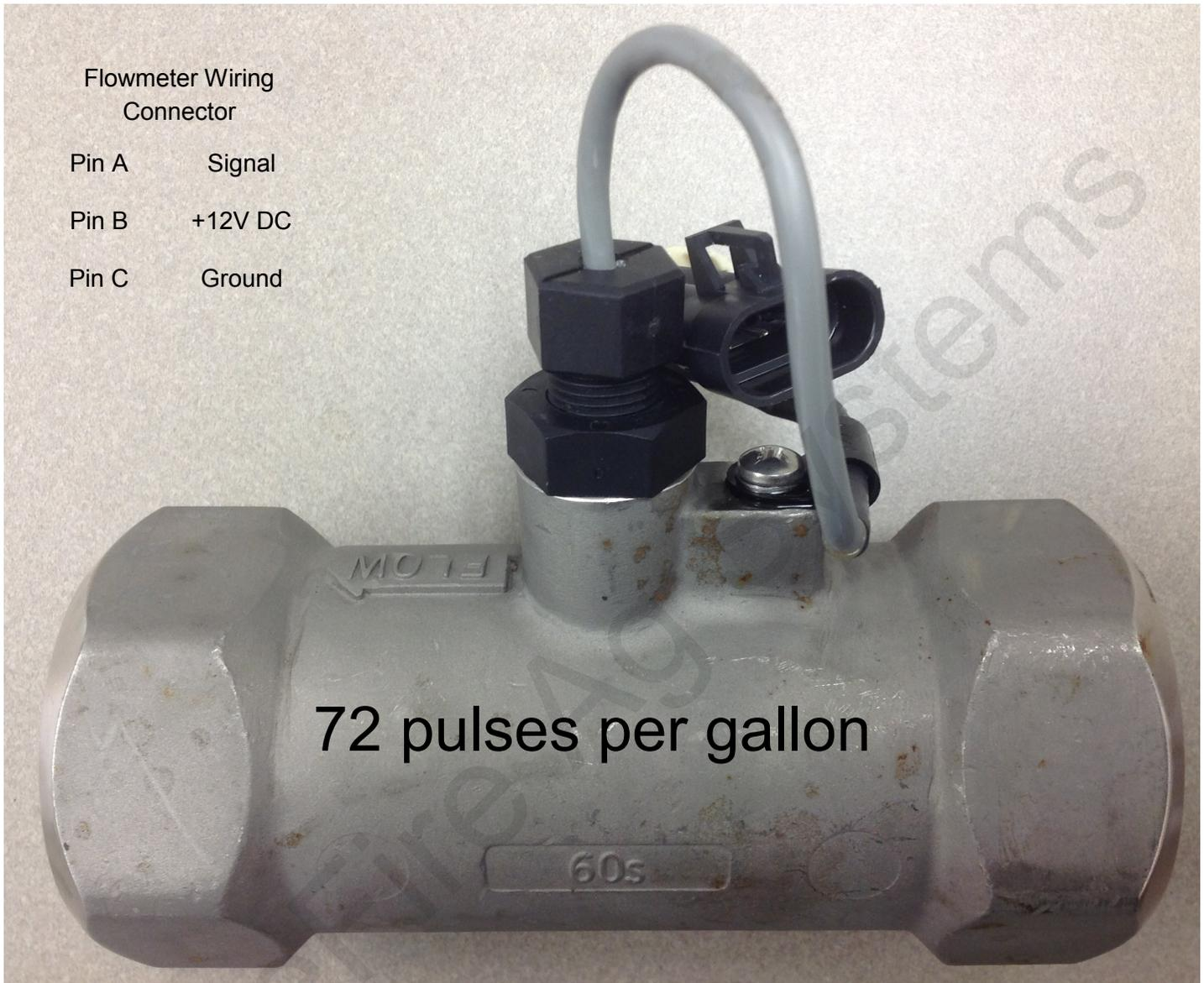
The flowmeter calibration number is **72 pulses per gallon**.
