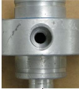
Threaded orifice not installed
