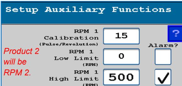
*(The SurePoint hydraulic pump with an RPM Sensor is 15 pulses/rev as shown)*
