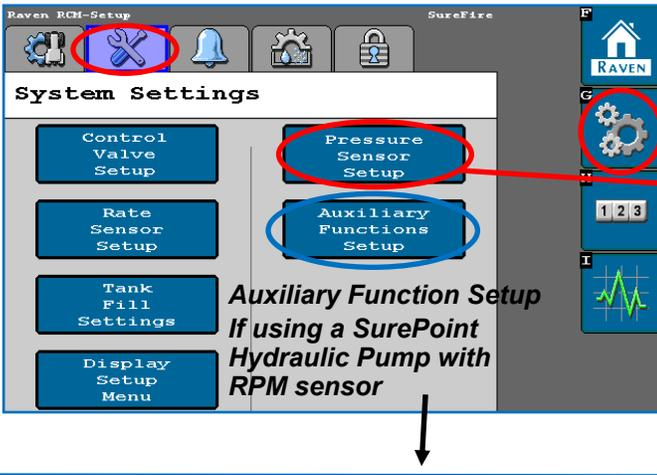
SurePoint recommends putting the Pressure Sensor reading in your **Display Settings** on the Run Screen (see next page). For complete information on how the sensor is operating, go to **Diagnostics > System Information > Pressure Sensors**. 0 Pressure Voltage should be 0.00 V.
