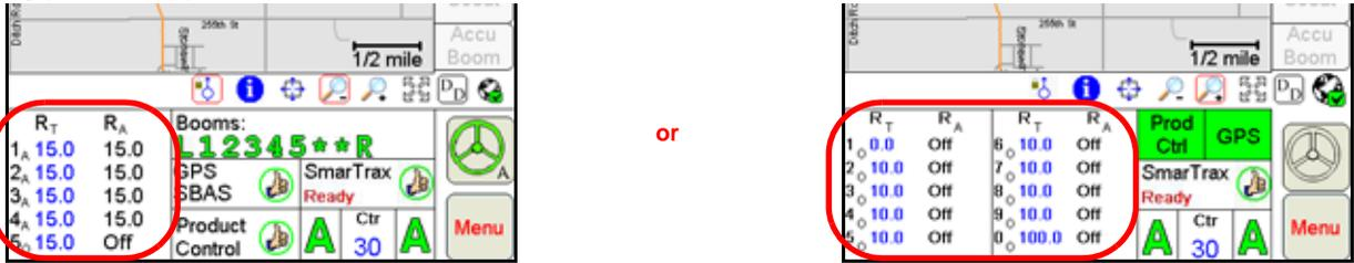
**Note:** The “Application Rates” heading will be hidden if multiple product nodes or control channels are enabled to allow all information to be displayed on the main screen.
