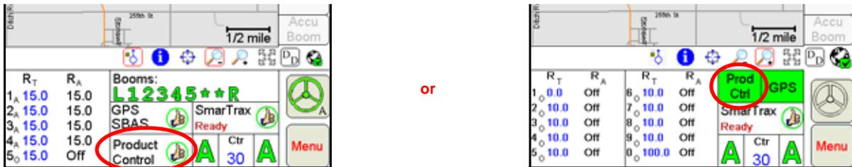
The status indicator displays a red 'X' if communication with the Raven serial control console or CANbus system is not available. A yellow 'caution' symbol is displayed if the Viper Pro detects a problem with the CANbus system such as an alarm condition. The status indicator will display a green 'thumbs-up' during normal operation.
