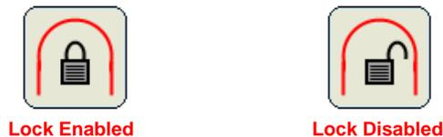
Touch the icon to toggle the turn around lock feature on to provide guidance back along the last swath and ignore the headlands area. Touch the icon again to toggle the turn around lock feature off to allow guidance along the headlands area.
