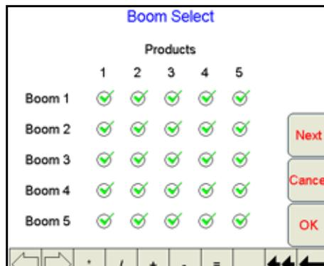
2. Assign products to boom sections as appropriate for the application equipment or system configuration. The system plumbing or configuration must be capable of the assignments shown on the Boom Select screen.
