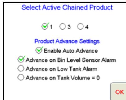
The nodes or channels assigned to the product chain during the job setup are displayed on this screen. The nodes are listed in the order that they will be used if 'Auto Advance' is left on. The settings are global for the
