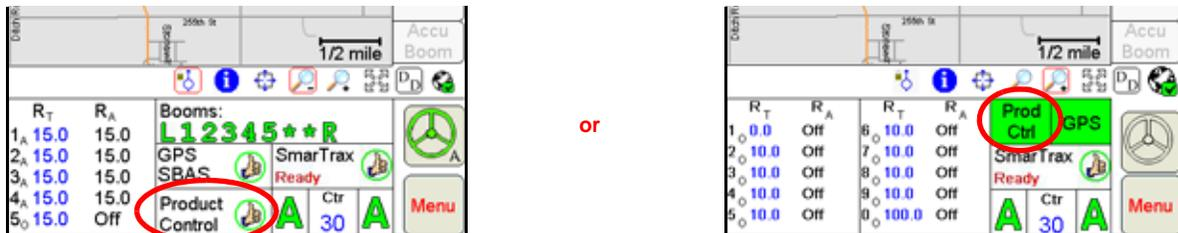
The Controller Status screen displays information from the product rate controller or a CANbus control system.
