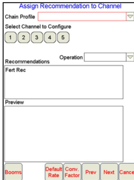
This screen displays the available control channels and any recommendations available for the selected field. If the Viper is controlling more than one product via a CANbus, the **Chain Profile** selection will be displayed at the top of the screen.
