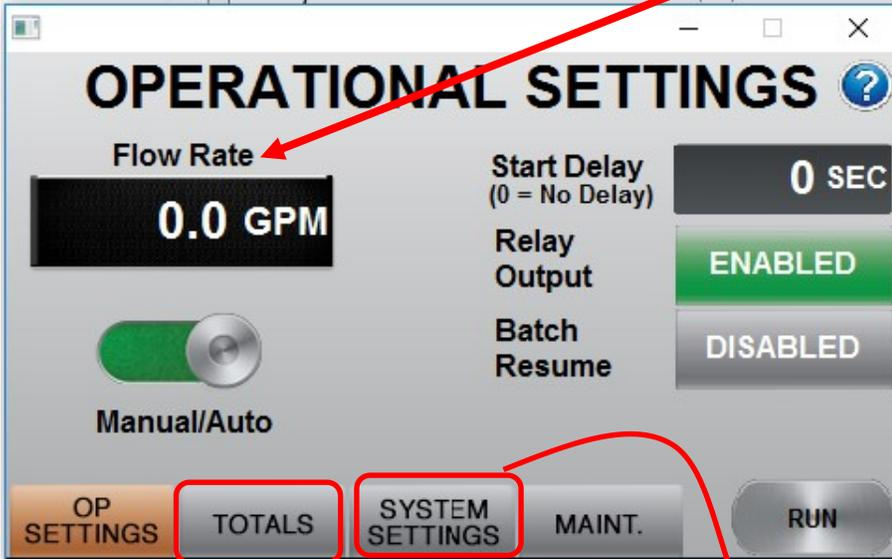
The **START DELAY** is used to delay the start of a batch by the number of seconds you enter.
