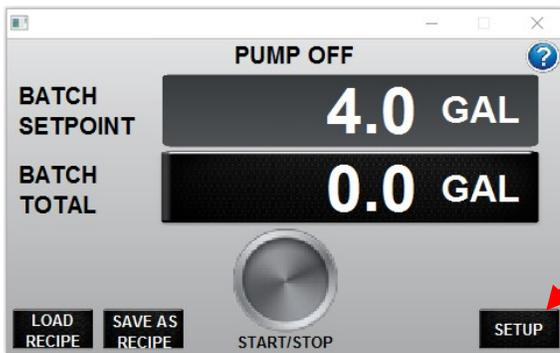
To get to the Operational Settings screen, press the SETUP button on the RUN screen.
