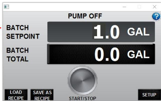
3. Hit the Start Button to start the catch test into the pitcher. Once the Test is done, the Batch Total should Read 1 GAL and the Pitcher should be at the 128oz level.
