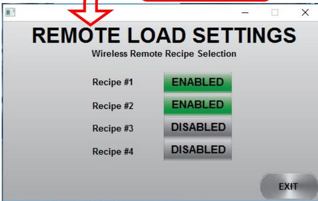
This screen sets if the #1-#4 buttons on the Push Button Remote Box or the R1-R4 Buttons on the Wireless Remote will select a recipe. As set here, #1/R1 button loads recipe 1 and starts the batch. #2/R2 does the
