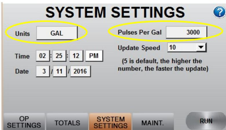
Press the System Settings button, Make sure "Units" is set to GAL and "Pulses per Gallon" is set to 3000. As shown to the left.
