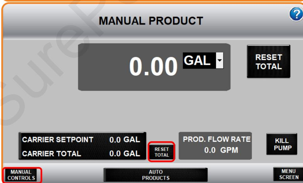
When a Carrier flowmeter is installed and enabled, the controller will count all carrier/water flow with the batch. **RESET TOTAL** after each batch. See settings page for carrier flowmeter setup.
