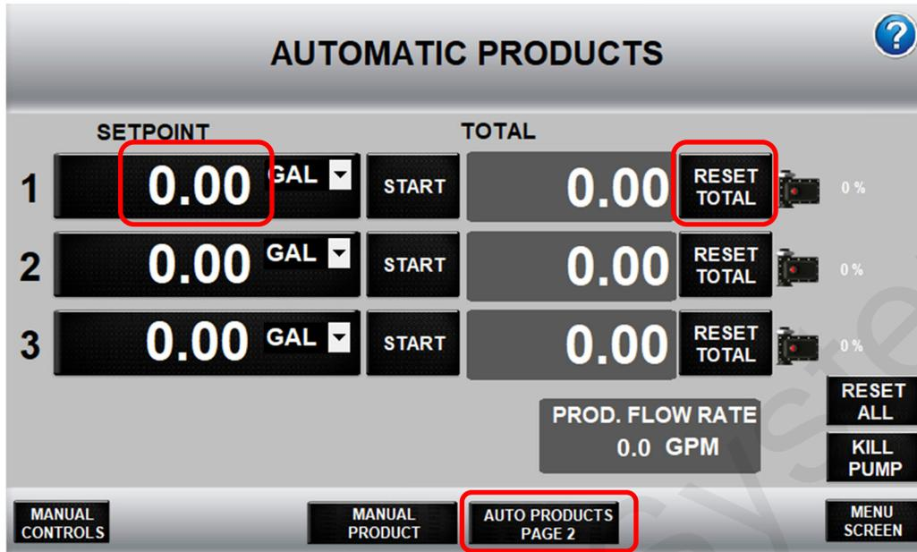
**AUTO PRODUCTS** allows the user to set the desired amount of product prior to the batch. Manually starting each product is still required.
