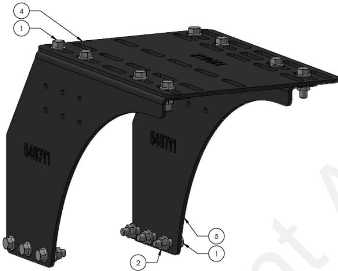
1. Mount 400-5467Y1 to the support plate using three (3) 1/2" x 1-1/2" flange head bolts and top lock nuts.
