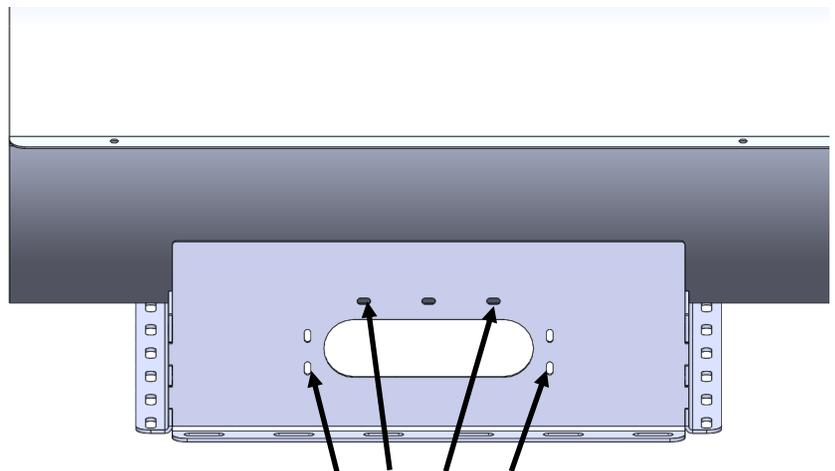
Bolt pump bracket through the slots on the side of the cradle.
