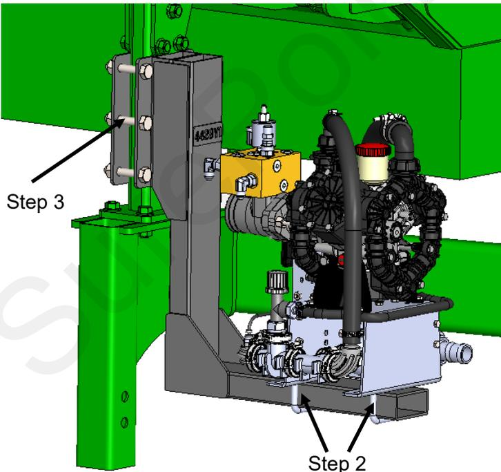
2. Mount PumpRight Pump on Horizontal bar of 410-4429Y1 Bracket using the supplied 1/2" U-bolts. Pump can be mounted 180 degrees from what picture on left shows per your preference on pump inlet and outlet locations.
