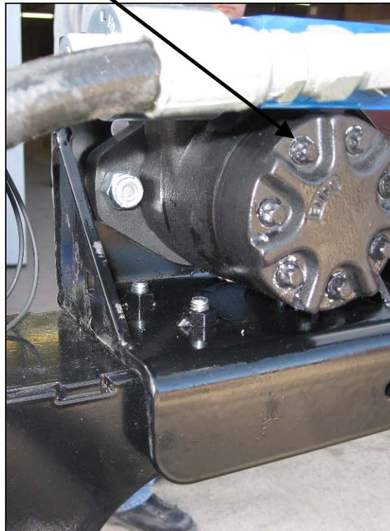
1. Hold all the motor sections together (3 plates).
