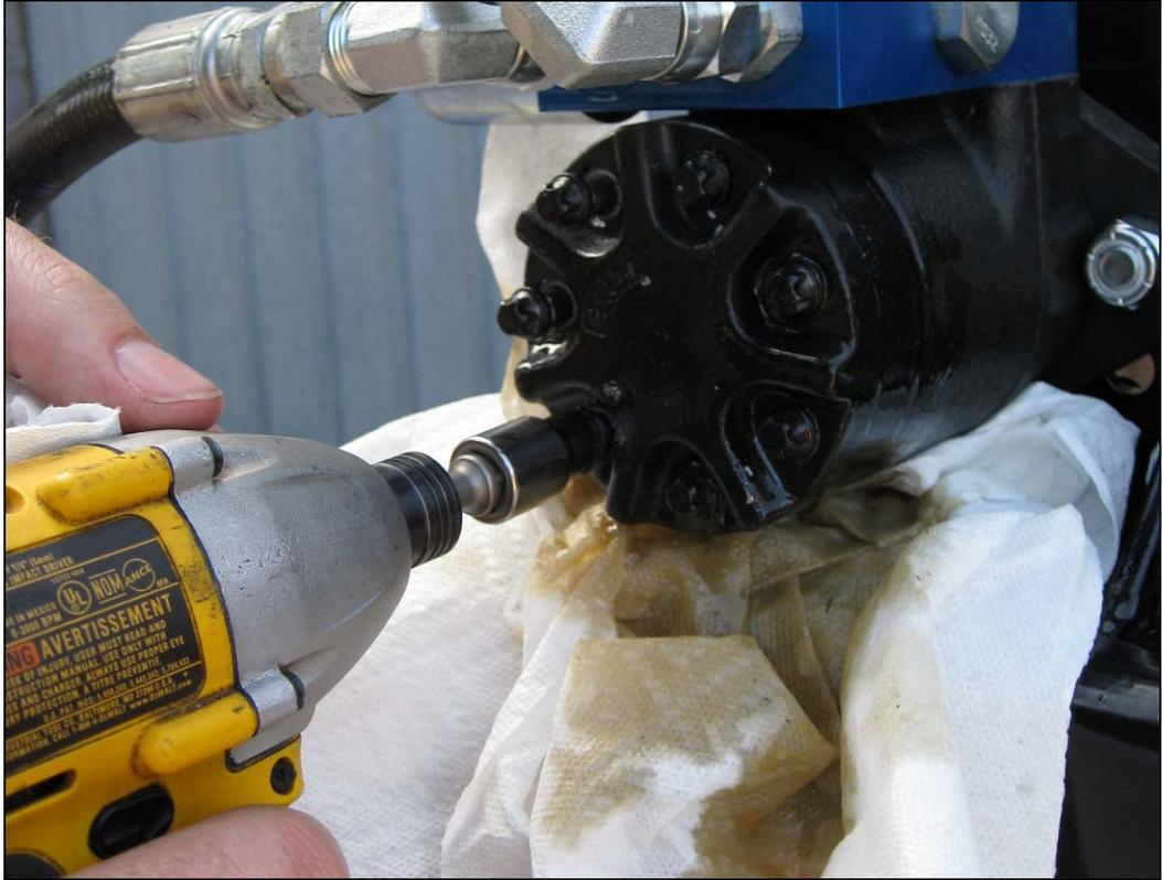
1. Reinstall and tighten the bolts evenly. Check the motor for proper rotation before connecting it to any other components which may be damaged.
