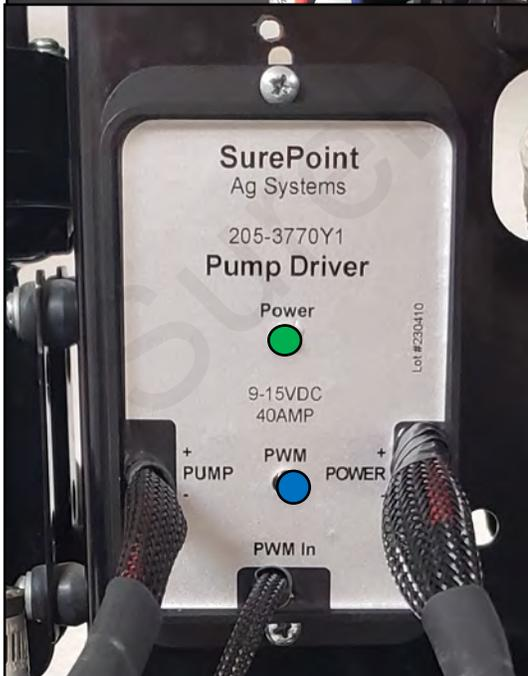
The **Green Power light** should be on when the EPD is receiving power from the battery.
