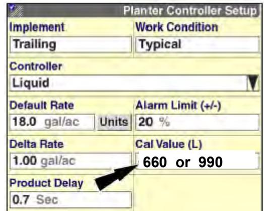
Refer to the AFS Pro 700 Planter Software Operating Guide or other Case IH publication for complete setup and operating instructions. Screenshots shown here are for typical liquid setups. Your setup may vary. Adjust as necessary in the field.
