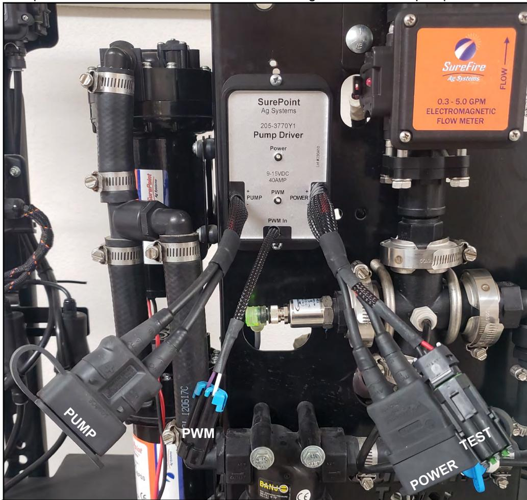
The **EPD** powers 1 or 2 electric pumps by providing a PWM (pulse width modulated) signal from the controller to control pump speed. It needs to have a power connection and wiring capable of carrying up to 40 amps of current. **It must be connected directly to the tractor battery.** SurePoint recommends 8 gauge wire (or heavier) if extending harnesses in the field.
