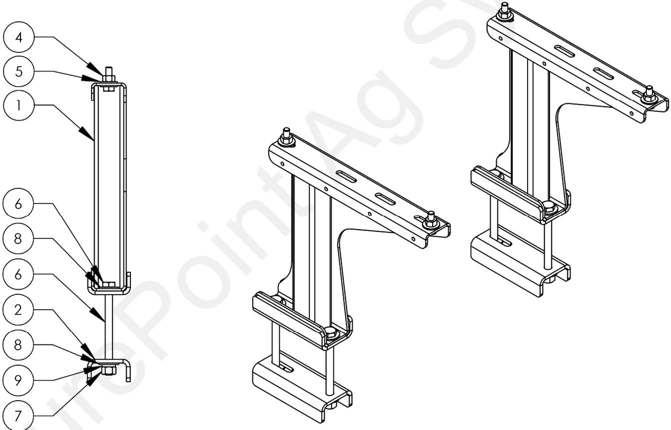
SurePoint Accelerator (55, 110 and 155 gallon) or Catalyst™ (55 and 100 Gallon) tanks can be mounted above and offset from a toolbar using this z-mount bracket. This kit attaches to 5" - 7" wide toolbars. The kit includes 3/4" x 9" bolts to work with a 7" tall bar.
