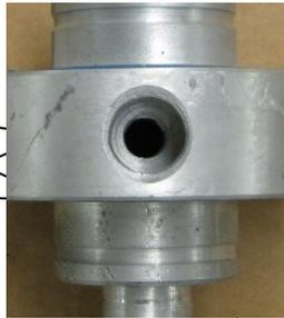
**Threaded orifice not installed**
