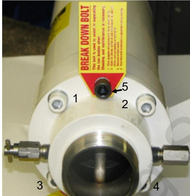
2. Replace both inner o-ring dump seals and body o-ring seal. Repair kit part number 153-01-A-SF-RK. Lubricate the O-rings before installing them in the Toppedo tube and torque the bolt to 35 ft-lbs.
