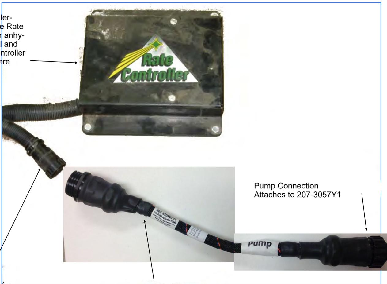
37 Pin Connector (on John Deere Harness)
