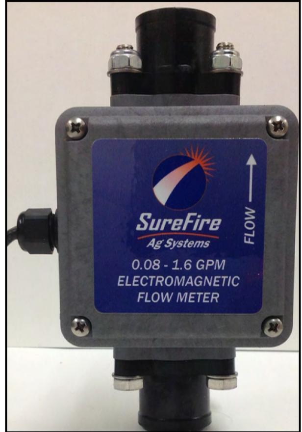
Electromagnetic flowmeters are superior to traditional turbine flowmeters in two basic ways. First, they have no moving parts. This translates into no wear items or potential for contaminants to jam a spinning turbine.
