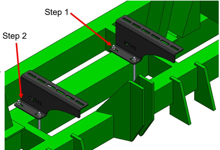
3. Position SurePoint Ag Torpedo bracket (PN 2719Y1, Not Included in Kit 516-04-150150) on 2821Y1 brackets. Bolt loosely using 1/2" hex head bolts and 1/2" flange nuts.
