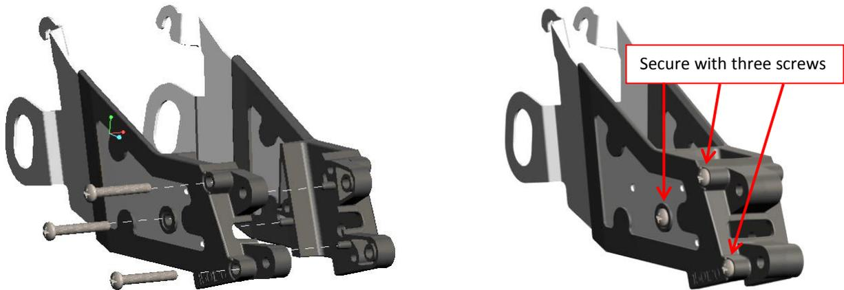
Illustration 2 – Assemble Quick Attach Firmer Bracket
