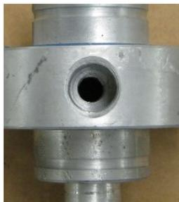
Threaded orifice not installed
