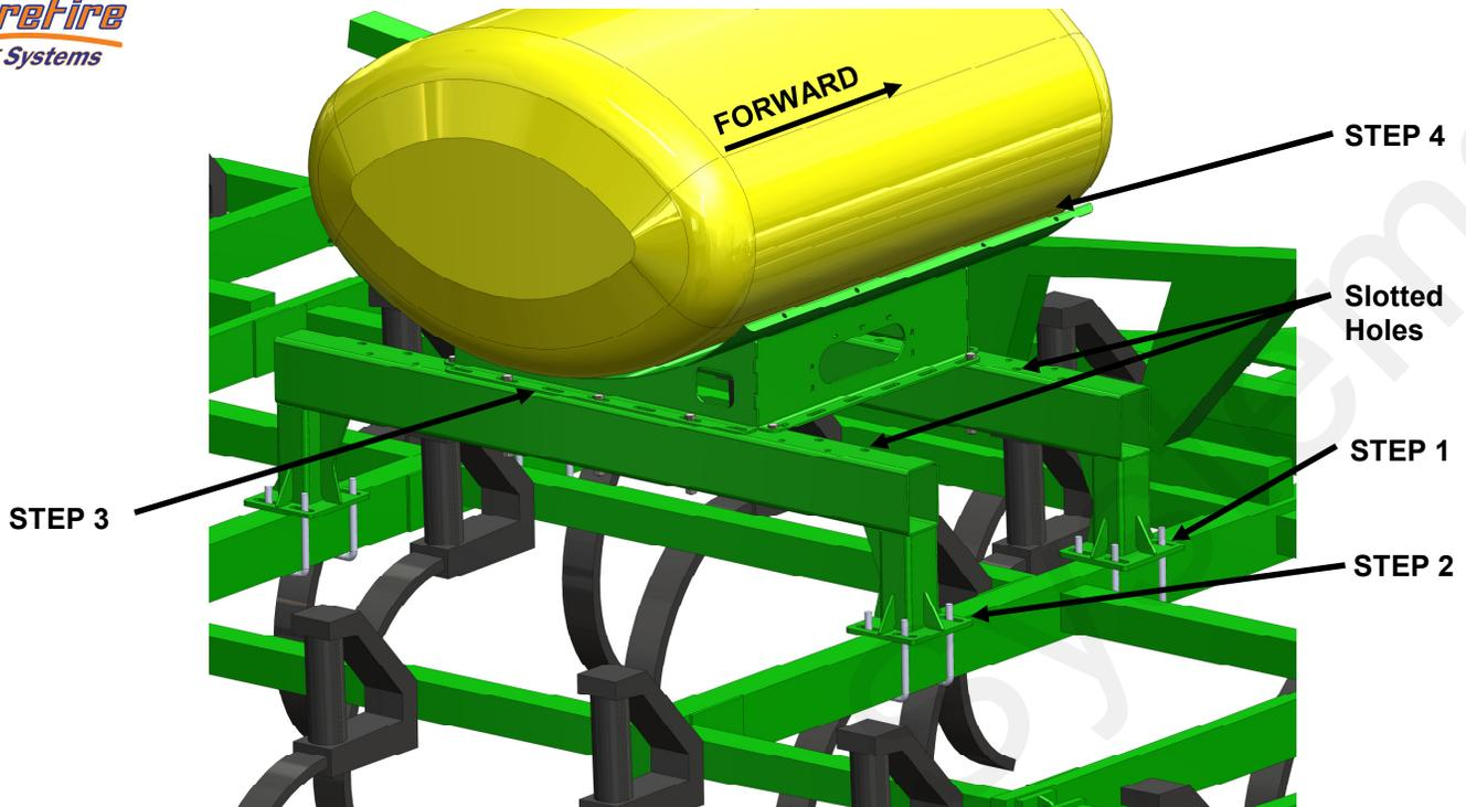
1. Mount the Front Tank Stand (420-2835Y1) with the supplied Square Bend U-bolts (380-1033) as shown in picture above. Refer to 'Detail A' below for approximate locations of where Tank Stand needs to be mounted per specific Tank Kit. **Make sure the slotted holes on the top of the Tank Stand are toward the Rear of the Implement.** Do not fully tighten U-bolts to allow for adjustment in Step 3.
