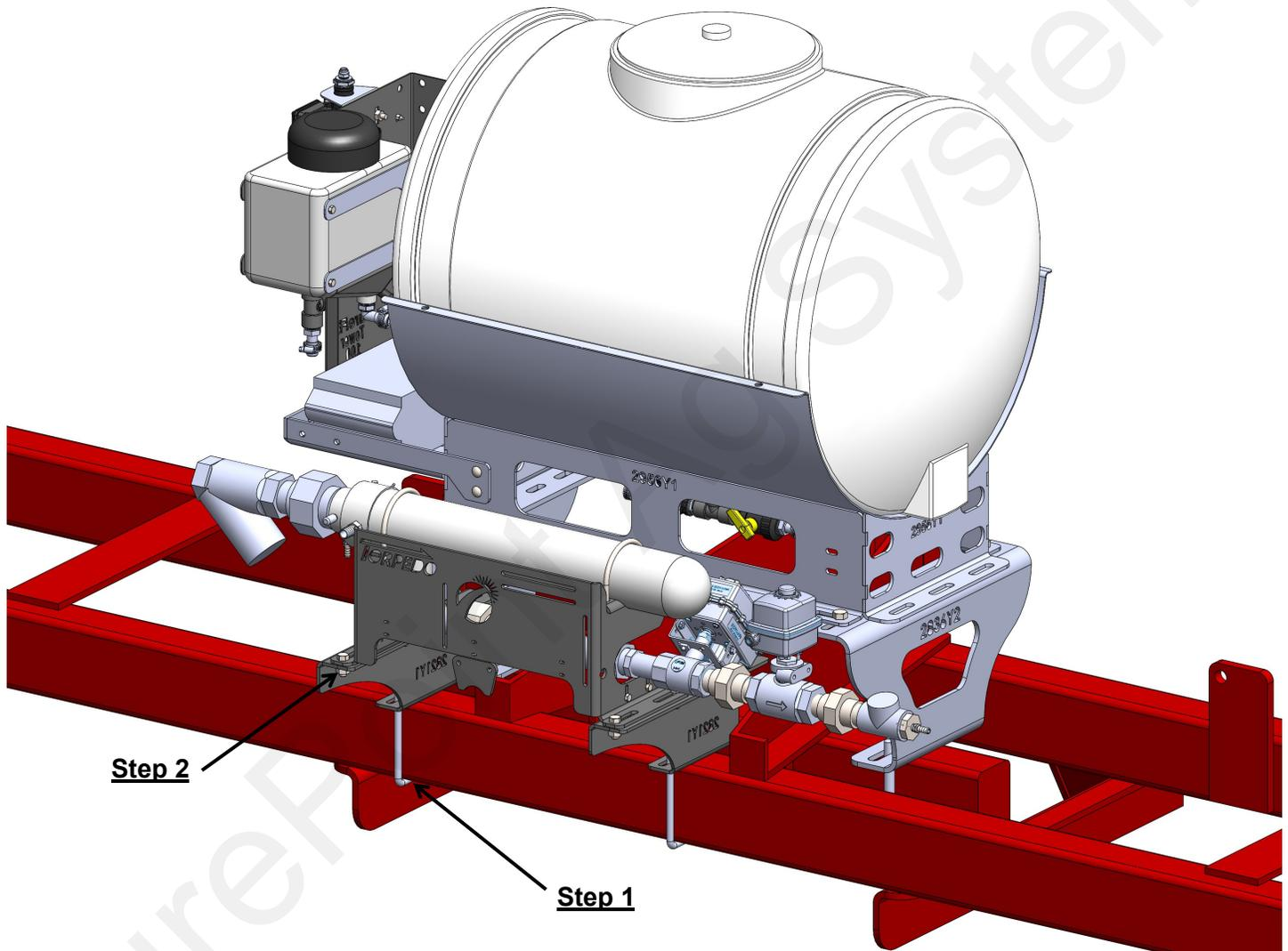
1. Mount the Offset Torpedo Mounting Brackets (462-2821Y1) to the the rear bar using the 1/2"x4"x7-1/2" Square Bent U-bolt kit provided (380-1015).
